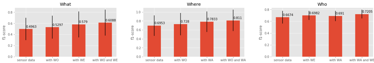
Figure 3. F_1 of our context recognition model. From left to right: perdurant (WA), enduring (WE), and social context (WO), respectively. The leftmost column refers to a predictor that uses sensor data only, while the other columns to predictors that in addition have access to context annotations.
