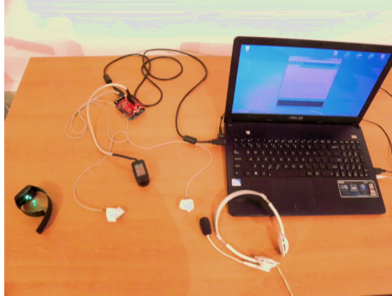
Fig. 2. Experimental setup, including of e-Health’s GSR electrodes and pulsioximeter for HR readings, as well as Empatica E4 wristband. In the latest studies conducted, either one of the e-Health of Bitalino platforms were used.
